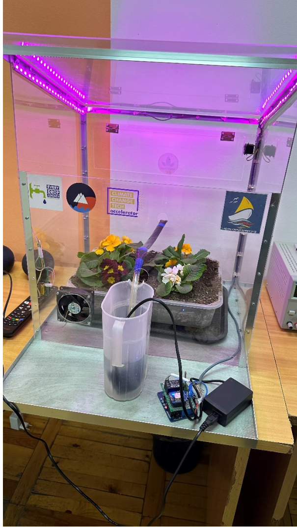
SmartHome demo model is based on Sonoff smart lights and smart power switch devices. SmartHome lighting system is integrated with Amazon Alexa and Yandex Alisa voice assistants.
